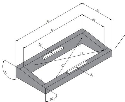
the upstand must be designed to be load-bearing all around and can safely absorb all vertical loads and horizontal spreading forces.
